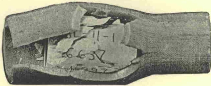
SOLID CYLINDERS OF SOLENHOFEN LIMESTONE
